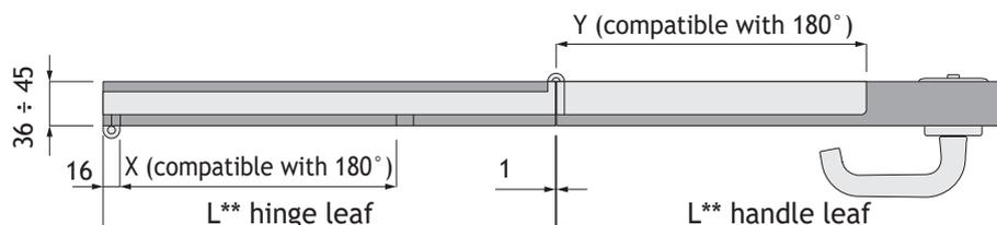
(\*\*) Hinge leaf and handle leaf widths are calculated with a reciprocal distance of 1 mm.
