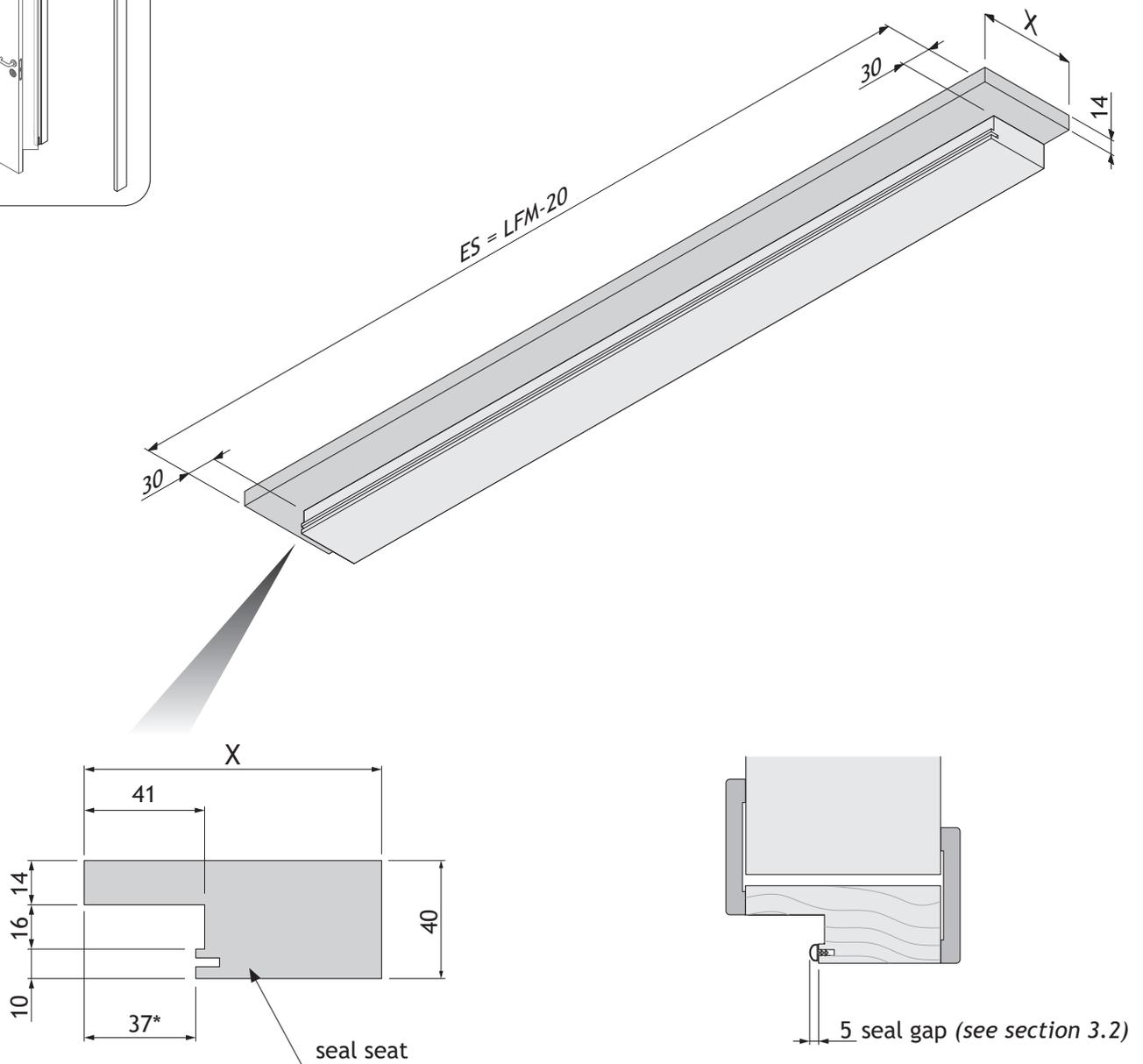
The dimension marked with (\*) vary according to the seal gap dimensions.
